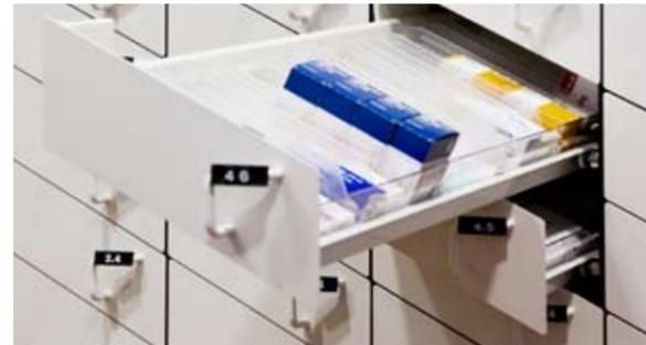
Refilling at the rear and picking at the front gives first in, first out stock rotation. The drawers handles are clearly marked.
