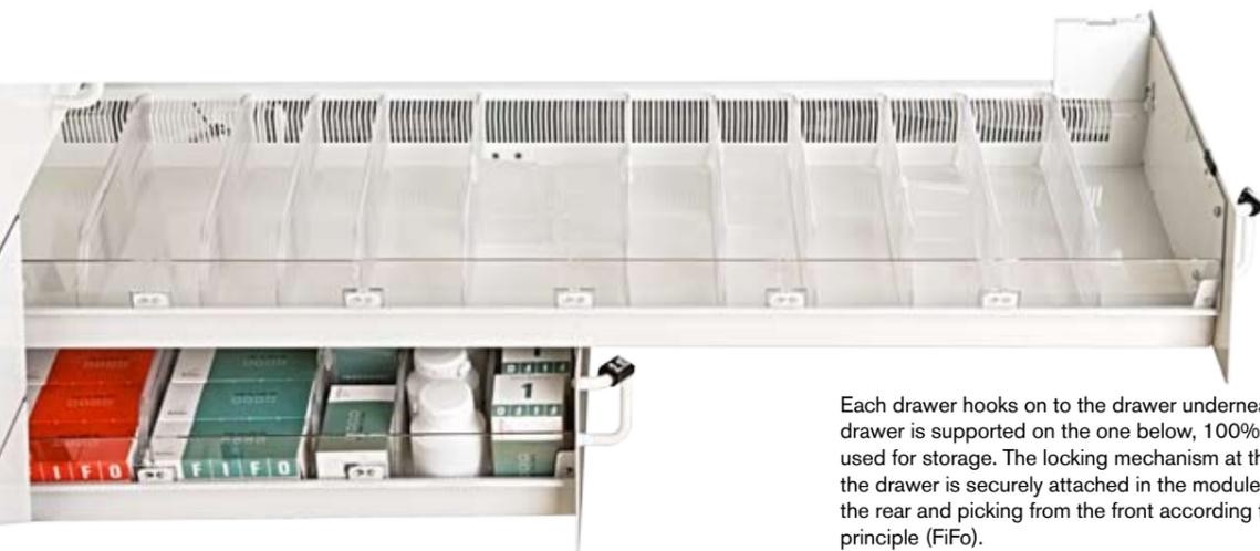
Each drawer hooks on to the drawer underneath. The pulled out drawer is supported on the one below, 100% of the drawer can be used for storage. The locking mechanism at the back ensures that the drawer is securely attached in the module. Refilling is made from the rear and picking from the front according to the first in, first out principle (FiFo).
